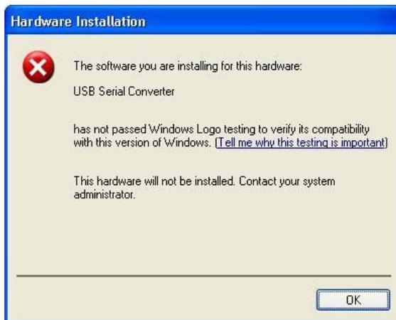
Two options are available to successfully install the device. Either a certified version of the driver can be installed (if available) or the driver signing options can be changed to either warn or ignore to allow the installation to complete. To change the current driver signing setting, go to "Control Panel\System", click on the "Hardware" tab and then click "Driver Signing". The desired signing option may then be selected.
