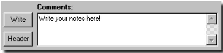
Pressing the **Header** button will display header in the Comments window. Pressing the **Write** button will save the displayed header in your current data file. Header contains the following information about settings of your measurements:
